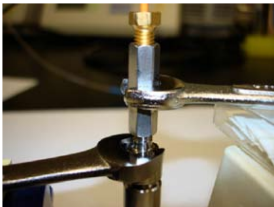
Figure 2: Installation of the pre-column tubing into the MassPREP Micro Desalting Column.
